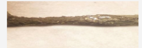
(c) Optical image of the file after electrochemical dissolution
