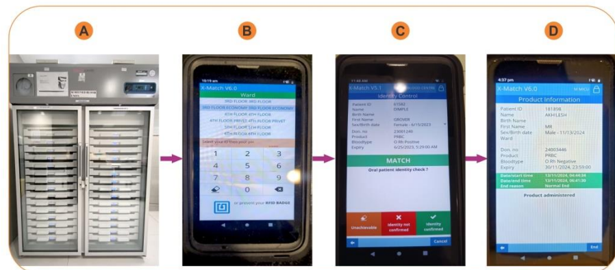
Process flow of RFID
